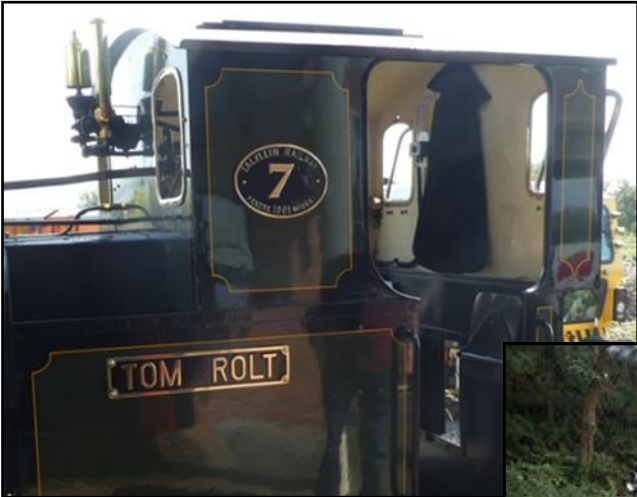
Talyllyn Railway. Locomotive No 7 named for Tom Rolt. 3 ft (914 mm) gauge 0-4-0WT well tank loco built by Andrew Barclay Sons & Co. of Kilmarnock in 1949, originally for Irish railways, acquired by Talyllyn Preservation Trust.
