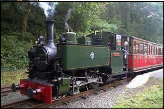
Talyllyn Railway. Locomotive No 7 named for Tom Rolt. 3 ft (914 mm) gauge 0-4-0WT well tank loco built by Andrew Barclay Sons & Co. of Kilmarnock in 1949, originally for Irish railways, acquired by Talyllyn Preservation Trust.
