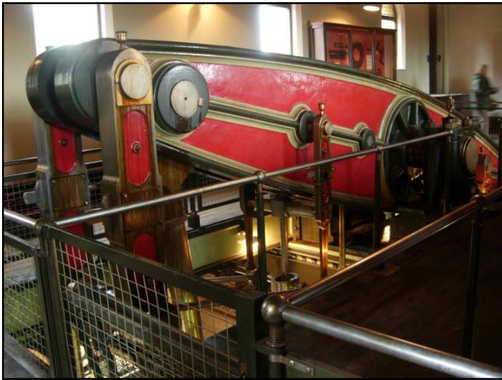
The 25ft. beam of one of the James Watt & Co. Engines
