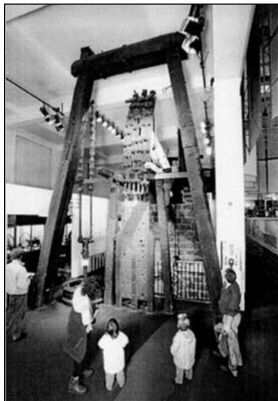
Newcomen Engine made at the Smith's Griffin Foundry in 1791 for Boulton & Watt, now in the Science Museum
